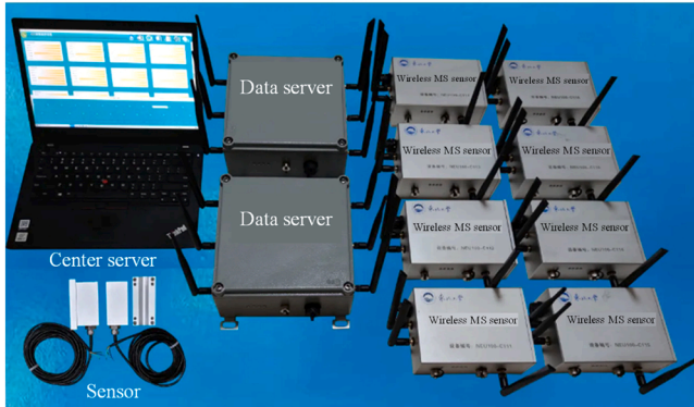
Fig. 16. The wireless MS monitoring system for rockbursts.
