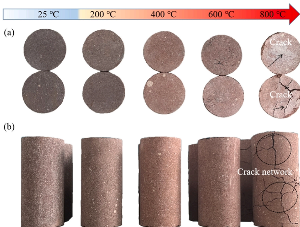
Fig. 5. Apparent color and crack evolution of red sandstone after high temperature.
