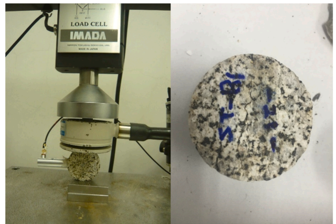
Fig. 8. Views of a Brazilian test and a tested sample.
