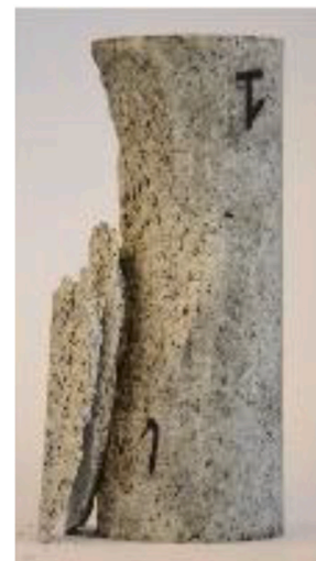
Fig. 19. The final failure mode of the granite specimen (50 mm in diameter with a length-to-diameter ratio of 2.5).
