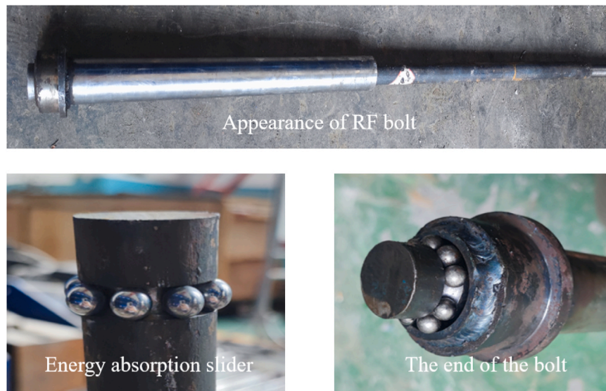
Fig. 3. RE bolt specimen for pull tests.
