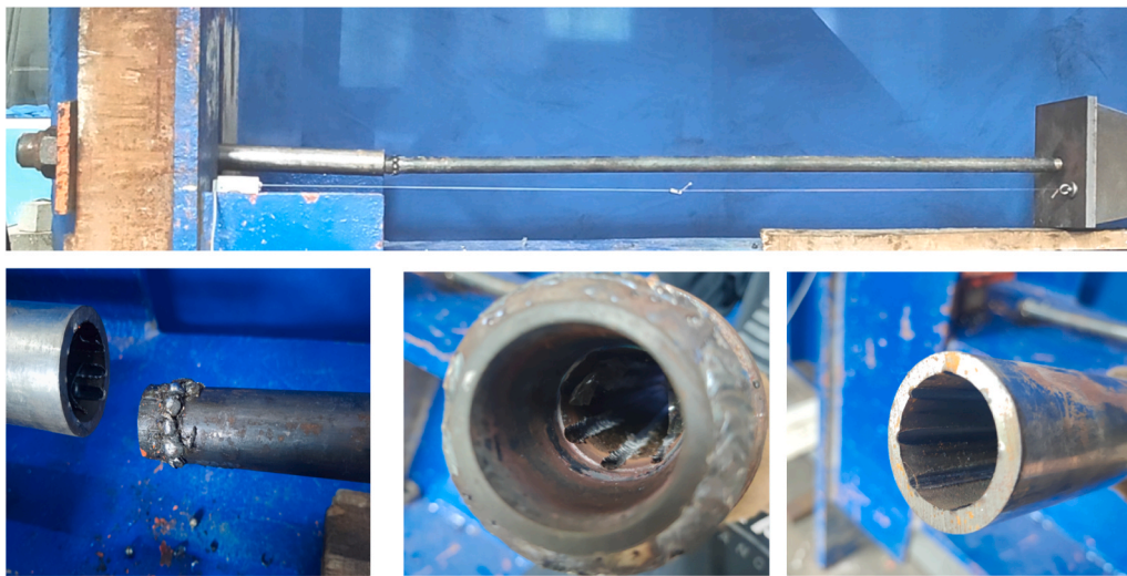
Fig. 11. Failure characteristics of the RE bolt.
