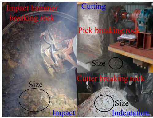
Fig. 1. Comparison of mechanical rock breaking slag size.
