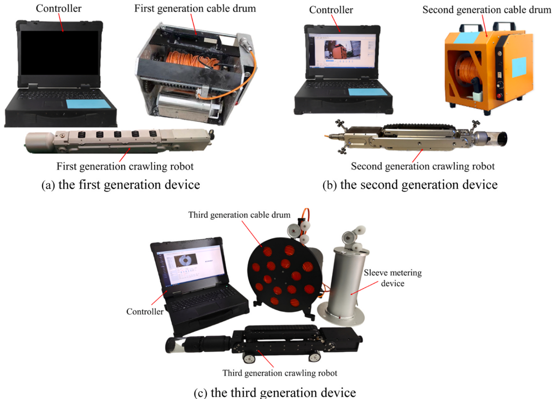
Fig. 1. An intelligent continuous monitoring device: (a) the single tracked monitoring device for hard rock fractures; (b) the dual tracked continuous monitoring device for hard rock fractures; (c) the dual track and wheeled integrated continuous monitoring device for hard rock deformation and fractures.
