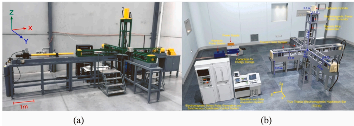
Fig. 15. (a) Photo of the triaxial Hopkinson bar system [15] and (b) the schematic of the TEHB system [141].
