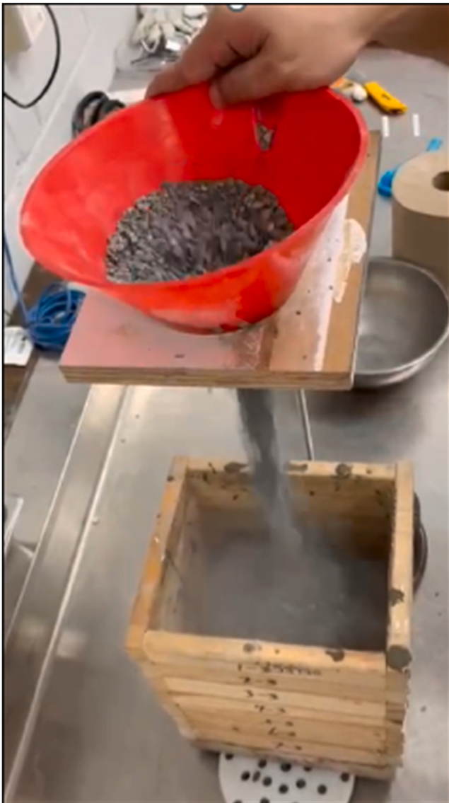
Fig. 15. A picture taken during the dumping of WR onto the PB for small-scale tests.
